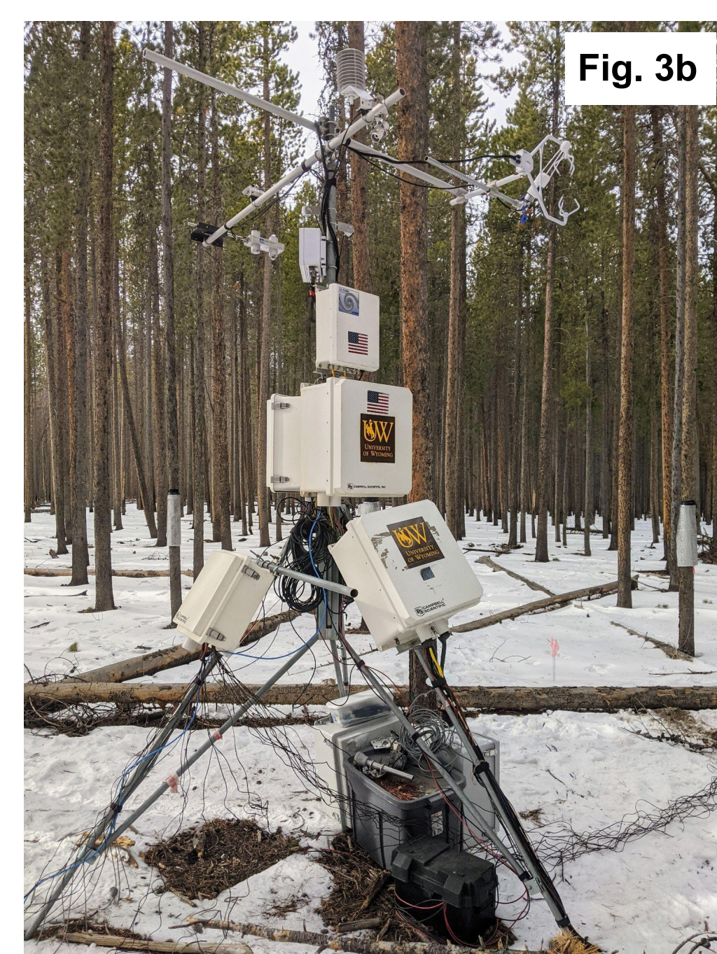
Fig 3: (a) The main 17m tower at US-CPK in 2020 (b) One of the three understory towers at US-CPK, which are deployed in unburned, severely burned, and understory-burned sites (c,d) Example timeseries showing the progression from winter (persistent snowpack, zero soil heat flux, below-freezing air temperatures) to snowmelt (isothermal/unstable snowpack, near-freezing air temperatures) to summer (no snow, fully thawed soil, warm air temperatures). Summer ends at first snowfall, winter begins at first persistent snowpack. (e,f,g) Energy budget plots using data from 2019 - 2022. Energy budget closure suffers during snowmelt as latent heat accumulates in the snow.
