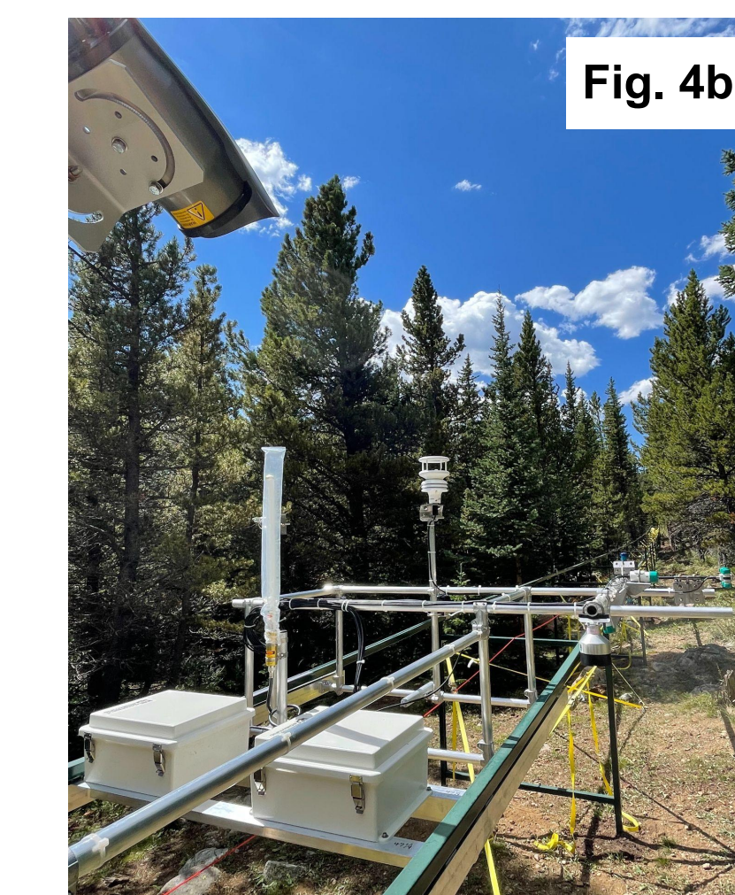
Fig. 4a. GPS units are placed above and below the canopy. Signal differences can be used to infer water interception. Fig. 4b. Tram-mounted instrument system runs between a mixed conifer forest and a perennial wetland
